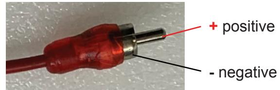
**Step 5)** Using a multimeter select OHM/continuity and put the leads on the RCA end and the stripped wire to determine which wire matches the center pin of the RCA connector.
