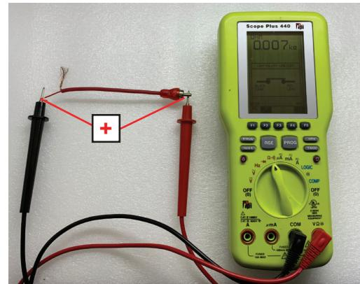
**Step 6)** Once it is determined which stripped wire is (+) positive and (-) negative you would wire that to your high output (speaker wires) from your source unit. Then make your solder connections.
