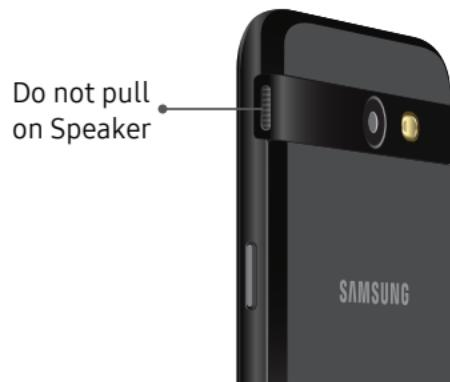
**Warning:** Do not bend or twist the back cover excessively. Using excessive force on the cover during removal or installation of an internal component can cause the material to break.
