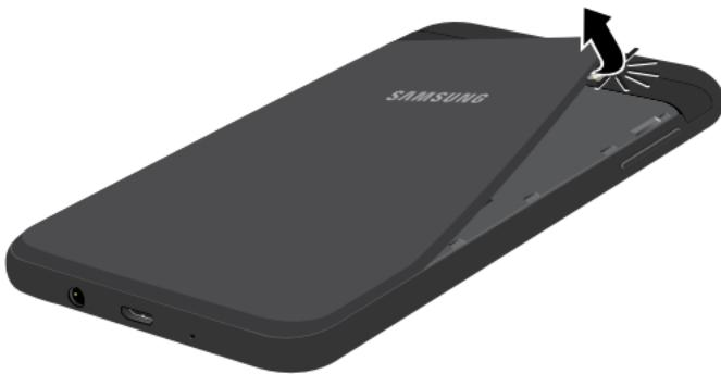
2. Lift the cover up and to the left of the device.
