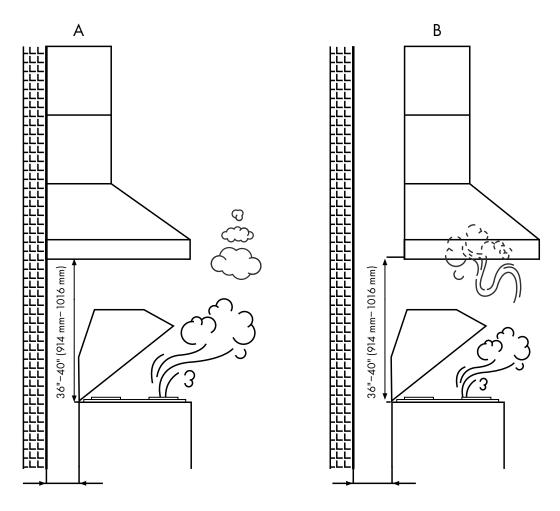
Smoke and hot air from an outdoor barbecue grill rises quickly, especially as the lid is opened. Not only does the smoke rise fast, but it is usually deflected forward (toward the cook) beyond the grill hood's capture area by the shape and position of the lid itself. Heavy, fast rising smoke is a challenge even for high-performance grill hoods, but there are some things you can do to enhance your outdoor hood's performance.
