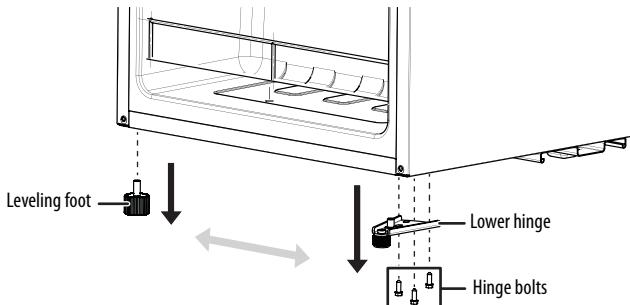
**9** Attach the lower hinge and leveling feet to the opposite sides of your cooler.
