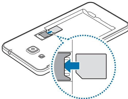
► **Dual SIM models:** Insert the SIM or USIM card with the gold-colored contacts facing downwards.
