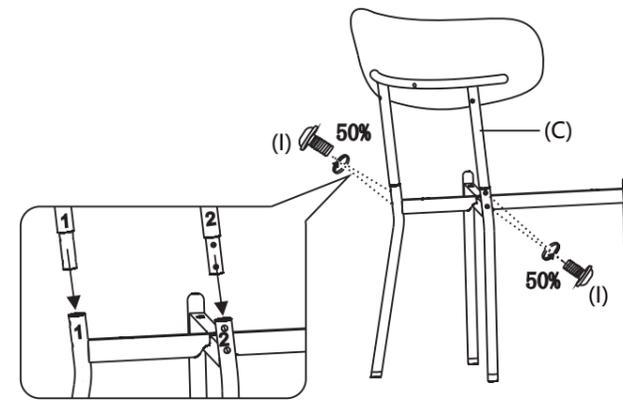
**3** **NOTE:** The bolts are only tightened 50%, When installing; please match the numbers on the backrest and legs.
