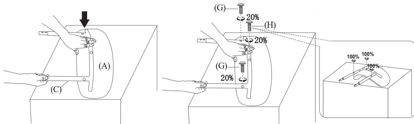
**1** Press down hard to fit Backrest Frame C and Backrest A, then align the holes to fix the Bolts G\*2 then Bolt H. First tighten 20% then tighten 100%.
