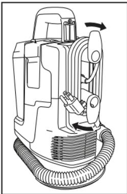
Wrap cord around the cord hooks for convenient storage. Attach the plug end to the cord.
