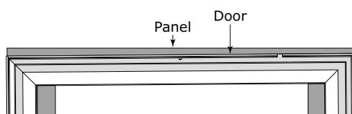
6. Secure integrated panel to door/drawer using clamps. A robust tape may also be used. U-Line recommends the use of bar clamps to secure the panel to the door/drawer. If using tape, be certain the tape will not damage panel finish upon removal.
