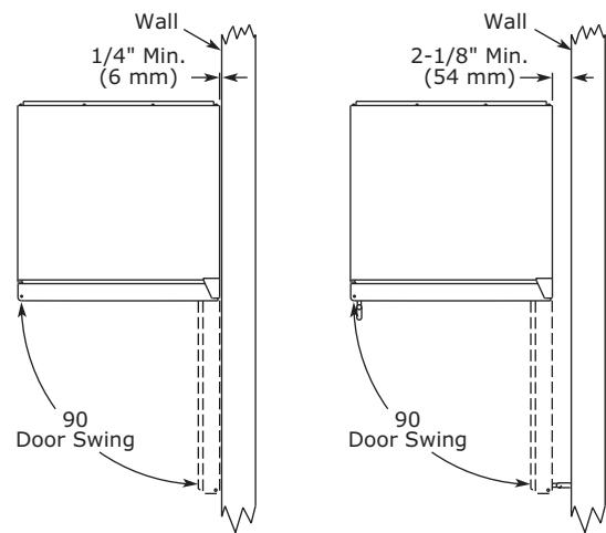
Units have a zero clearance for the door to open 90°, when installed adjacent to cabinets.
