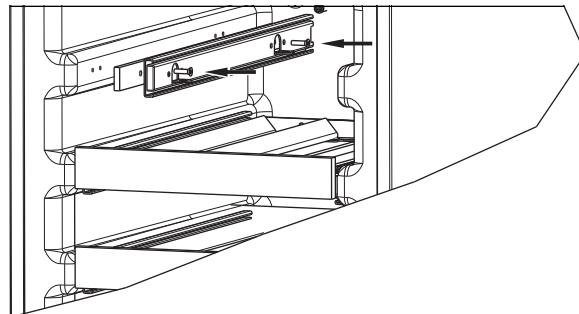
2. Starting from the side that has the spacers (previously unaltered units will be on the right hand side from the factory), remove 2 screws, slide and spacer.
