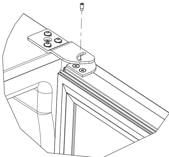
3. On 24" models, a second pin is included for the bottom hinge. Repeat steps above for second hinge.
