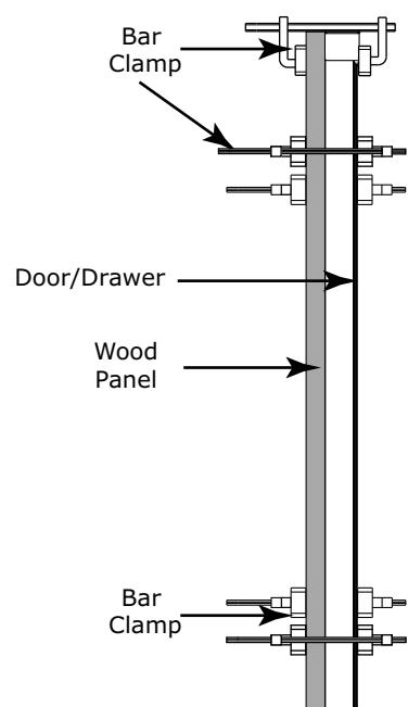
7. Using a 7/64" (3 mm) drill bit, drill 6 pilot holes into the wood panel 1/2" (12 mm) deep using the holes in the door/drawer frame as a guide.
