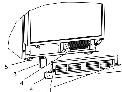
**When using the unit, the grille (plinth strip/base fascia) must be installed.**
