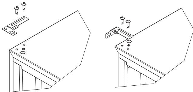
3. Place bracket (part #14154) over holes and attach to unit with two screws removed in step 2 using a T-25 Torx driver. Tighten screws fully.
