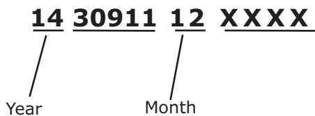
A typical serial number is shown above. The first two digits of the first segment, 14, represents the production year. The number between the dashes, 12, represents the production month. In most cases, warranty status can be verified by the production date information within the serial number.
