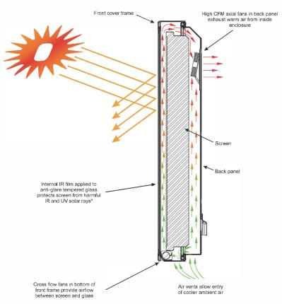
\*To maintain the effectiveness of the anti-glare glass and maintain picture quality, the screen must be mounted so that the front of it is between 0.75 in. and 1 in. from the glass.
