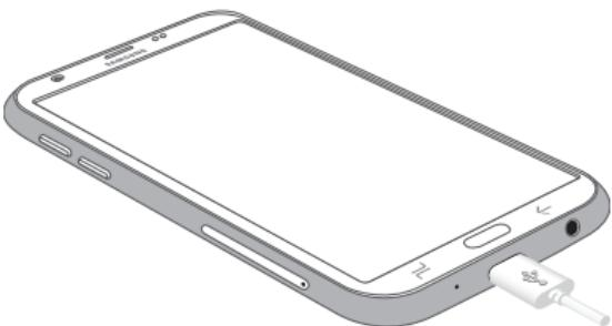
2. Connect the USB cable to the charging head, and then plug the charging head into a standard outlet.
