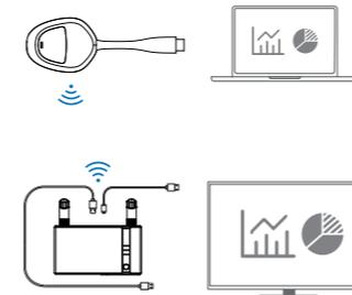
1. Connect the HDMI port or VGA port of the receiver to the video input port of the display device (monitor or TV).
