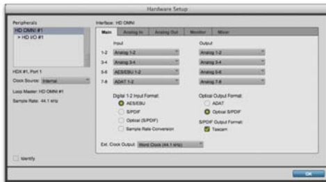
Hardware Setup for HD OMNI, Main page
