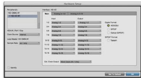
HD I/O Hardware Setup, Main page
