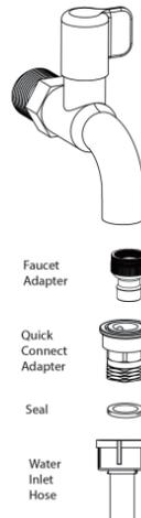
**If water leaks from faucet connection or washer connection, turn off water and tighten fully using a wrench. Be careful not to over tighten and damage water connection. Turn on water supply and make sure no leaks are present.**
