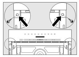
Use the screws supplied to secure the microwave oven to the side walls of the cabinetry through the holes in the oven trim.
