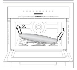
■ To remove the turntable, press down on one side (1.) and lift it up by the other (2.). Wash the turntable in the dishwasher or by hand with a weak solution of dish detergent.
