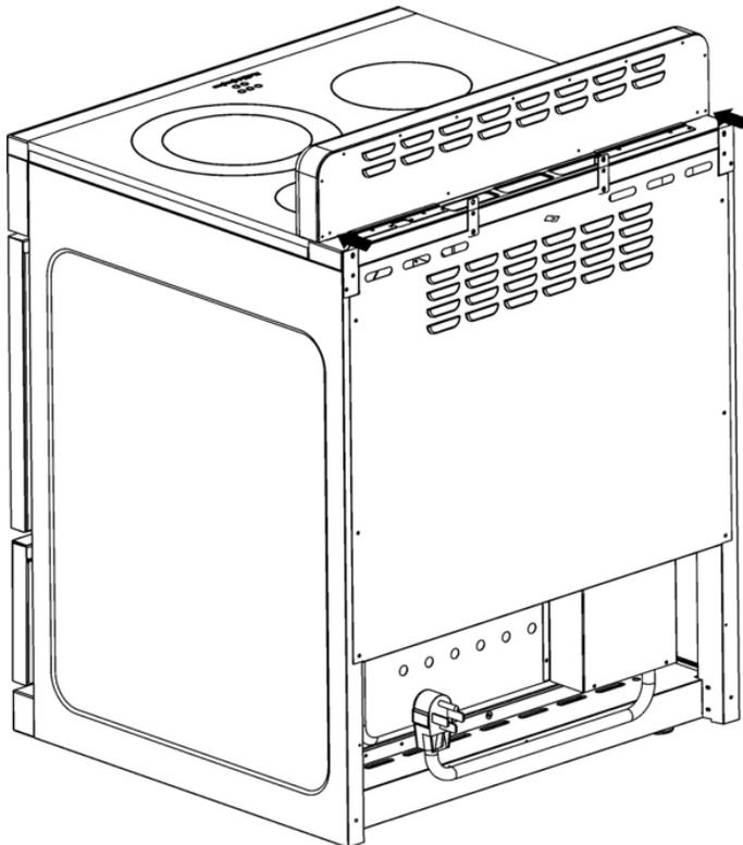
2. Secure the backsplash to the cooktop from the back using the 4 Phillips head screws provided as shown in the diagram.
