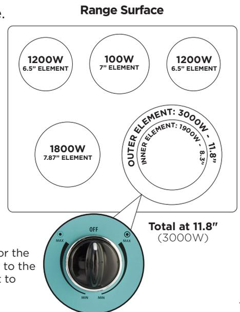
**NOTE:** Rotate to the left for the small element 8.3". Rotate to the right for the large element to add 11.8".
