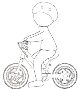
3. When the E-bike begins to glide, press the accelerator continuously. Put both feet on the pedals as desired.
