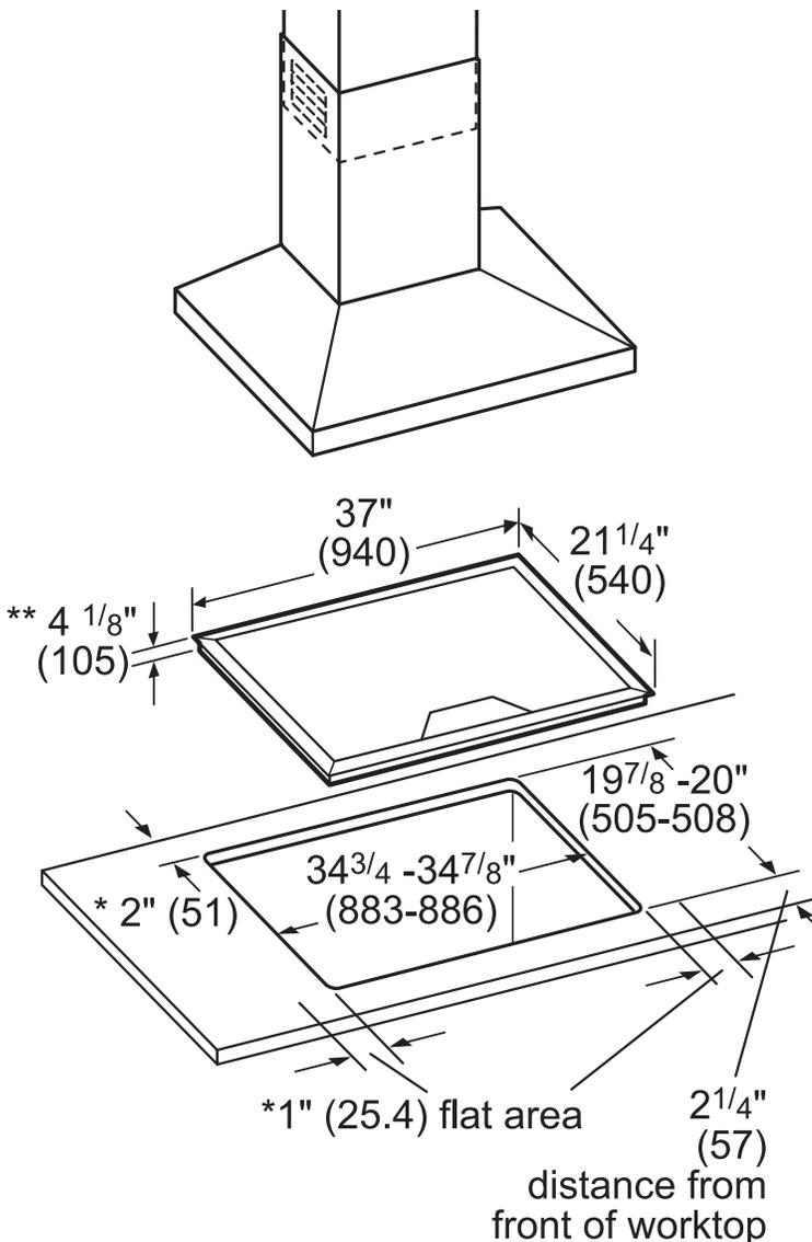
**NOTE:** The work surface should be horizontal and level. The stability of the countertop should be confirmed even after making the cutout.
