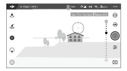
After confirming the selection, the aircraft will fly in the direction marked by the "GO" icon. The aircraft will automatically adjust its speed when it senses an obstacle out in front or if it is flying too close to the ground. However, this feature should not be relied upon for navigation between obstacles.
