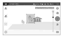
4. The aircraft will automatically avoid obstacles in its flight path. If the aircraft loses track of the subject, because it is moving too fast or is obscured, re-select the subject to resume tracking.
