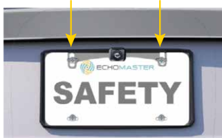
Camera mounts behind license plate
