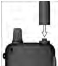
To connect the antenna, just screw it onto the SMA connector at the top of the scanner.
