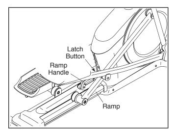
To lower the ramp, press the latch button, pull the ramp handle, and lower the ramp to the desired incline level. Then, release the latch button and engage the latch pin into one of the adjustment holes in the frame. Make sure that the latch pin is firmly engaged in one of the adjustment holes in the frame.
