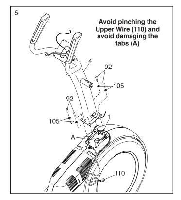
See the inset drawing. Locate the wire tie (B) in the lower end of the Upright (4). Tie the wire tie to the Upper Wire (110). Then, pull the upper end of the wire tie until the Upper Wire is routed through the Upright.
