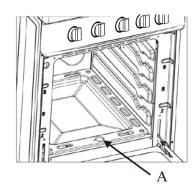
3) Press the knob inward and hold to activate the electronic ignition. Note that you will hear a "clicking" noise. Hold the knob pressed inward until the oven burner is lit. Keep the button pressed down for a minimum of 15 seconds before releasing it.
