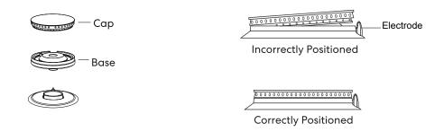
Check that the electrode is always clean to ensure trouble-free sparking.
