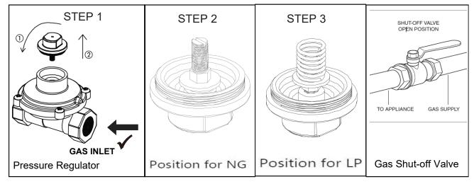
Pressure regulator can withstand a maximum input pressure of 0.5 psi (3.5 kPa), and is set at 5" WC outlet pressure when used on NATURAL GAS and 10" WC outlet pressure when used on LIQUID PROPANE.
