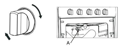
3) Press the knob inward and hold to activate the electronic ignition. Note that you will hear a "clicking" noise. Hold the knob pressed inward until the oven burner is lit. Once the oven burner is lit, release the knob.
