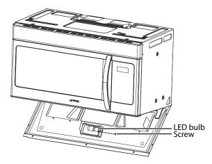
4 Swing the base plate back into place and secure it with the screws.
