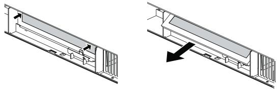
5 Slide the new filter into the top of the unit, then press the bottom of the filter into place.
