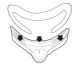
2. Attach the foam pad to the facial interface bracket via velcro®
