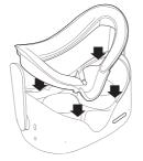
3. Align and pull the facial interface bracket to the Oculus Ouest 2.
