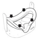
4. Gently press the facial interface bracket to secure it firmly on the Oculus Ouest 2.
