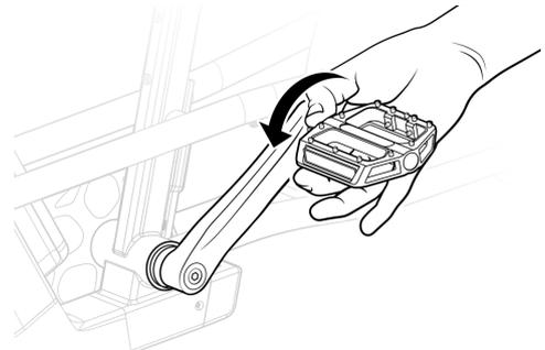
Thread the left pedal onto the left crank gently by hand, turning counterclockwise.
