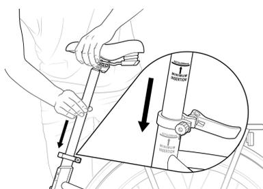
Insert the seatpost, ensuring the minimum insertion point goes into the seat tube.
