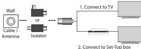
Connect one end of the isolator to cable/antenna jack and the other to TV set or set-top box.
