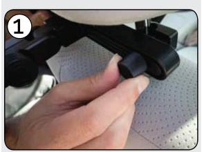
Loosen the thumb screws on the post mounts enough to allow the mounts to fit over the headrest posts.
