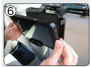
Insert the tablet by placing the bottom side against one arm grip, then swinging the top into position.
