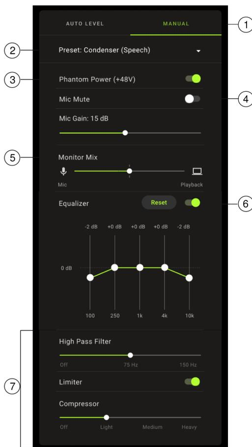
① **Auto Level Mode / Manual Mode** AUTO LEVEL mode allows the app to select best choices for your recording needs. Or select MANUAL mode for full control over the microphone settings.
