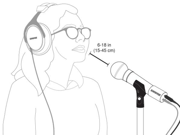
Ideal when the sound source is further from the microphone, like in gaming when the person needs to be closer to the screen or gaming console. Aim the microphone directly at the sound source. Place the microphone 6 to 18 inches (15 to 45 cm) away from the sound source. Make additional gain adjustments if necessary.
