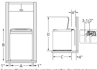
To ensure sufficient clearance for water lines and airflow, allow minimum clearances
