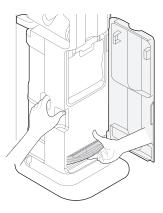
5 Remove dust from the motor protection filter and exhaust filter once every 3 months and wash it using room temperature water.
