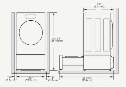
To ensure sufficient clearance for water lines and airflow, allow minimum clearances of at least 1 in. (2.5 cm) at the sides and 4 in. (10 cm) behind the unit. Be sure to allow for wall, door, or floor moldings that may increase the required clearances.
