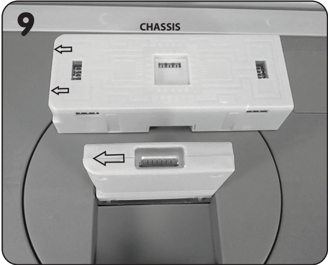
Use the included blueprints to build your vehicle. The chassis will always be the base of each vehicle. The arrows on the chassis and the chassis holder should face the left. Vehicle parts are interchangeable and can be assembled with most of the included tools.
