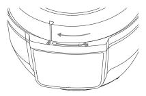
For pressure cooking, the lid will automatically lock when the multi-cooker starts building pressure.
