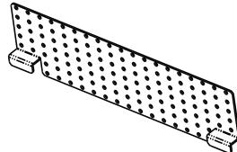
The anti-tip bracket has holes set up on a grid in order to better locate a wall stud. At least 4 places must be used.
