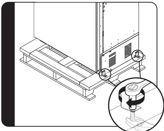
Remove shipping brackets from skid by removing four bolts (two on each side) with a 1/2" (1.3 cm) deep-well socket wrench and a pair of pliers. **Note:** Tilting unit is not required to remove shipping brackets.
