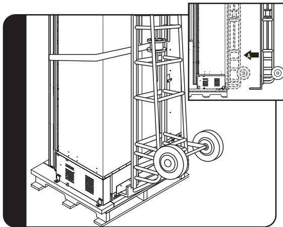
Slip appliance dolly between unit and skid. Remove unit from skid. **Note:** Use excess packaging to protect decorative trim; also, verify that leveling legs are up (0" adjustment).
