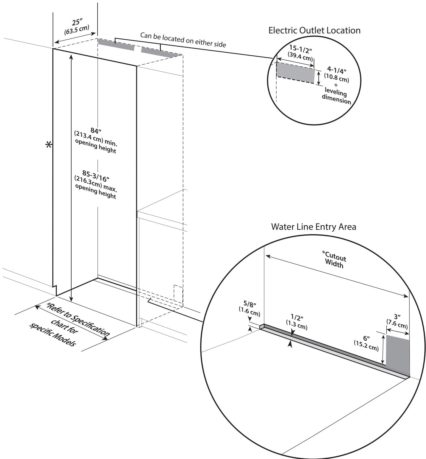
*\*Note: For all models, 3" back from the front of the cabinet on both sides needs to be finished like the outside of the cabinets*
