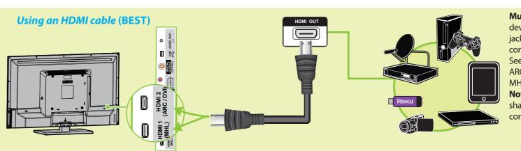
Multi-purpose jacks: You can plug any device that uses HDMI into either HDMI jack. However, certain devices must be connected to the ARC/DVI, or MHL jacks. See the instructions that came with your ARC, DVI, Roku Streaming Stick™, or MHL-enabled device for more information. Note: The HDMI 2 (ARC/DVI) jack is a shared jack. This means you can only connect one DVI or ARC device at a time.
