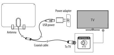
1 Plug the USB power cord into the power adapter, then plug the power adapter into a wall outlet.
