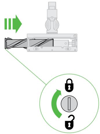
Mini motorized tool: Clearing obstructions
