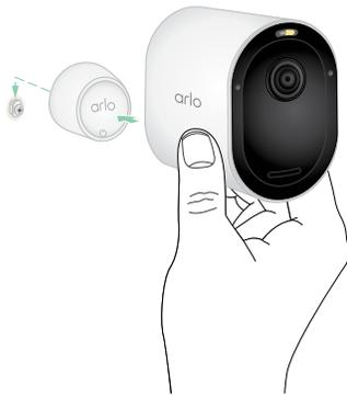
5. Attach your camera to the wall mount. The magnet in the mount holds the camera onto the mount.
