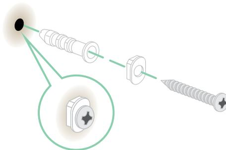
\*At 6.5 feet (2 meters) or higher, we recommend using the Arlo Outdoor Mount.
