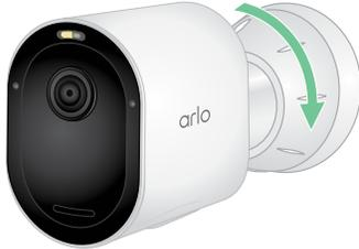
**Note:** To release your camera from the housing, insert the security key in the security keyhole and turn the key clockwise.
