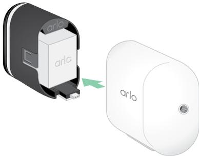
3. Pull the camera all the way out of the camera housing.
