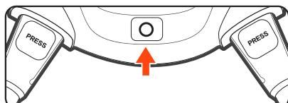
**STEP 3:** Lift the TYPHOON H PLUS airframe straight and level. When the LEDs on two motors start to blink green as illustrated, turn it forward as shown by the red arrow until a tone is heard and the two LEDs turn off.
