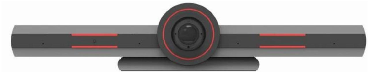
The Avaya IX CU360 camera is equipped with two rows of lateral LED strips on the front with a circular crown of LEDs around the camera lens. The LEDs display different colors and animation effects based on the camera status. The camera supports zooming the video from the web interface and the remote control unit. When the camera is zoomed in, you can also digitally pan and tilt the camera.
