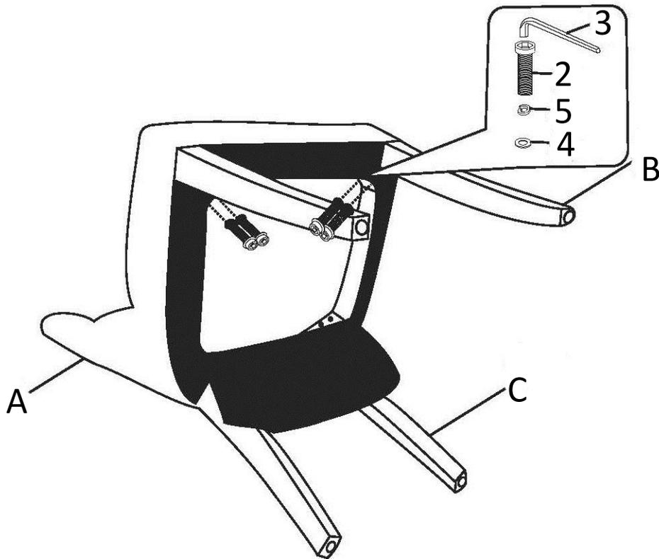
Attach Front Legs (B) to Chair (A) using Allen Key Screws (2), four Flat Washers (4) and four Lock Washers (5) into pre-drilled holes. Use Allen Key (3) to tighten. Do not over-tighten.
