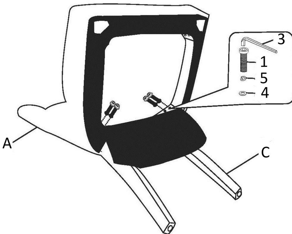
Attach Back Legs (C) to Chair (A) using Allen Key Screws (1), four Flat Washers (4) and four Lock Washers (5) into pre-drilled holes. Use Allen Key (3) to tighten. Do not over-tighten.
