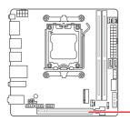
PCI\_E1: PCIe 5.0 x16 (From CPU)
