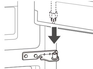
**2** Fit the hinge (1) over the hinge lever latch and slot it into place. Rotate the lever (2) counterclockwise to secure the hinge.
