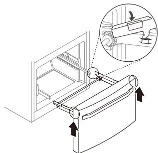
4 Insert the drawer into the frame, and push the drawer back until it clicks into place.
