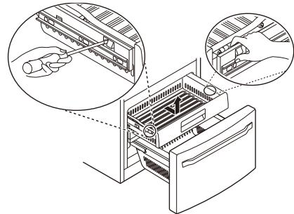
4 Remove the Durabase basket from the rails. Remove the screws from the rails at both ends.
