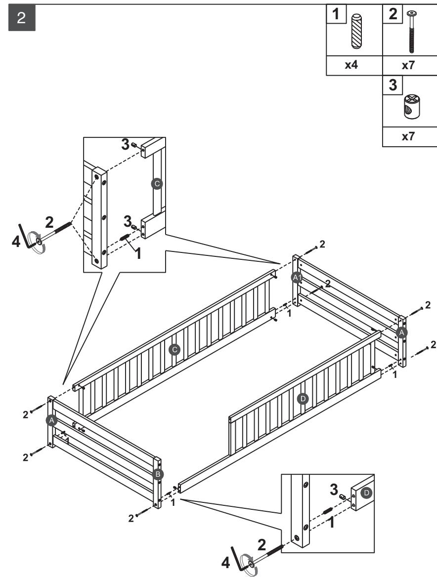
**EN: Note:** Part 3 will face up with the "x" mark on it, otherwise it cannot be tightened.
