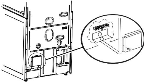
3. Remove plastic tag holding three 10-32 hex nuts from the middle post of the terminal block.
