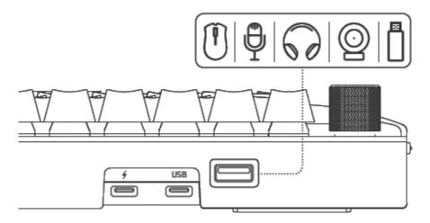
1 Not compatible with devices that require higher voltages or USB 3.0, such as external hard drives.
