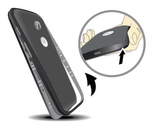
2. Pry the band off to expose the card slots.
