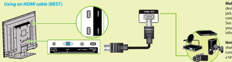
Multipurpose jacks: You can plug any device that uses HDMI into any HDMI jack. However, certain devices must be connected to the HDMI/DVI (ARC) I jack. See the instructions that came with your ARC or DVI device for more information.
