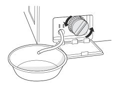
**5** Clean the pump filter and opening.
