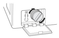
Close the drain pump filter cover.
