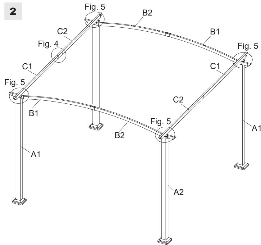
**EN:** Fig.4: Insert Connector Tube (G) to Lintel (C1) and Lintel (C2), make sure the holes are aligned. Then use Bolt (AA) to connect Lintel (C1), Lintel (C2) and Connector Tube (G).
