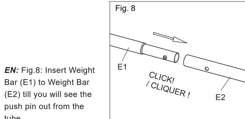
**EN:** Fig.8: Insert Weight Bar (E1) to Weight Bar (E2) till you will see the push pin out from the tube.
