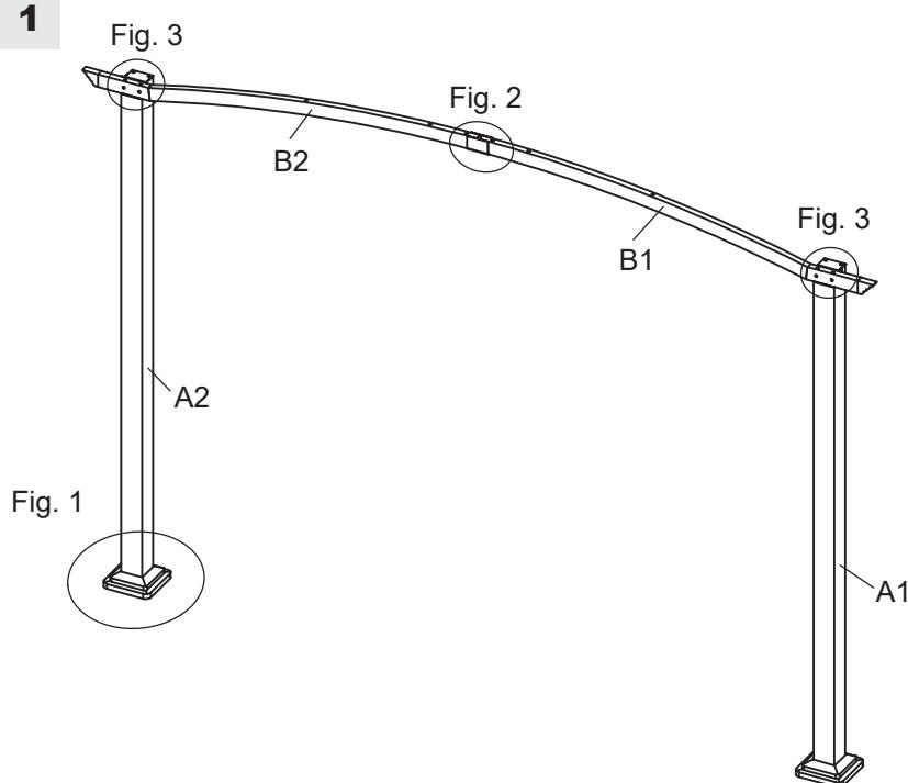
**EN:** Fig.1: Insert Post(A1) to Base Plate Cover (J), then using Bolt (AA) to connect Post (A1 & A2) and Base Plate (H). Repeat each step for A1/A2.
