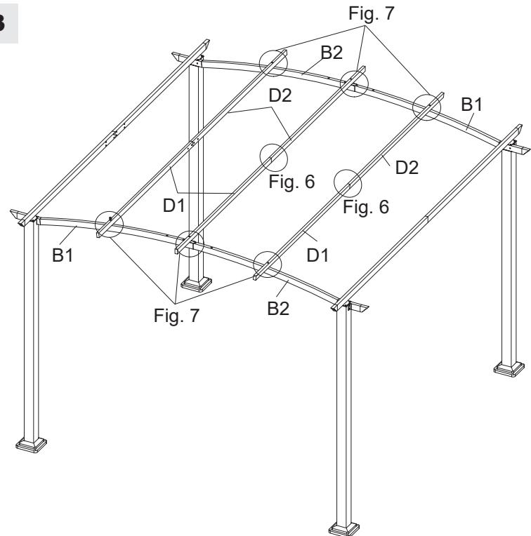
**EN:** Fig.6: Use Bolt (AA) to connect Roof Tubes (D1 &D2).
